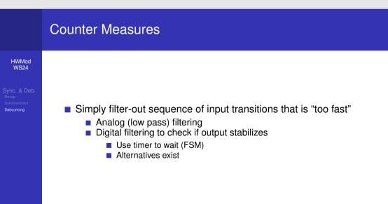
Simply filter-out sequence of input transitions that is "too fas a Analog (tow pass) fibering Digital filtering to check of output stabilizes Use time to waik (FSM) a Alternatives exist Software-based debouncing
