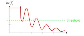
Asynchronous inputs are not the only problem at interfaces Some mechanical contacts may "bounce" due to their constructio ■ For example: Mechanical buttons, switches ■ Instead of clean transition dampaned oscillation
