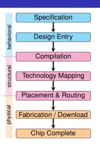
verbal / formal description of behavior model in description language (e.g., VHDL) translation to network of generic logic elements mapping to cells of target technology placement and interconnection of cells physical implementation
